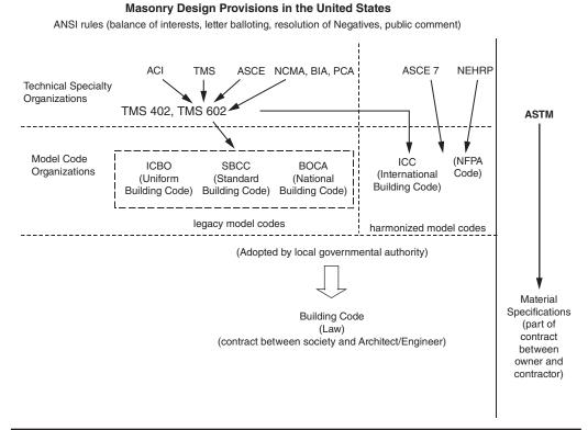
FIGURE 3.1 Schematic of process for development of masonry design codes in the United States.
