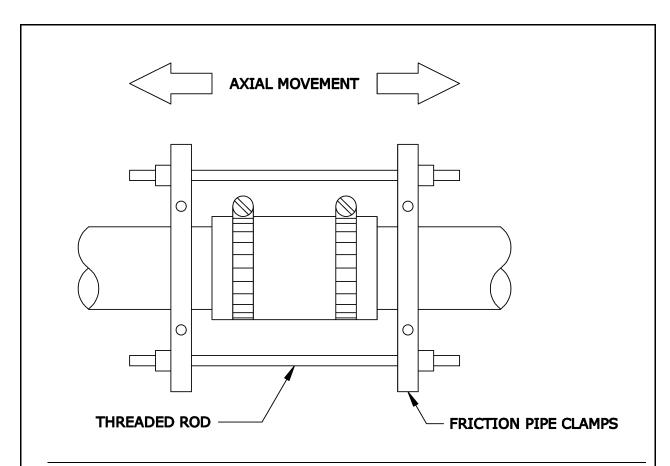
Although mechanical couplings using elastomeric seals are most often the type of joint to experience damage that is due to axial movement, this restraint requirement applies to changes in direction for all types of piping that exceed 4 inches in diameter.
