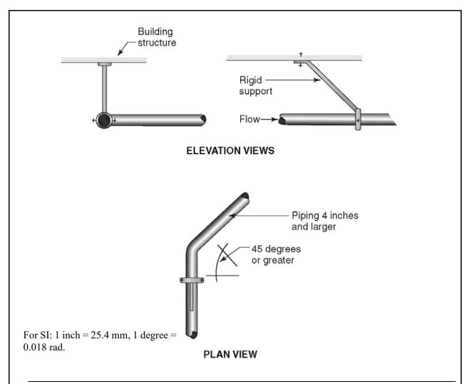
Sway bracing is installed to resist side-to-side movement of horizontal piping at a change in direction. A change in horizontal direction of 45 degrees or less is not considered significant enough to cause pipe movement.
