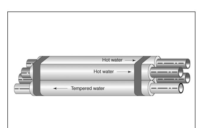
To prevent thermal transfer, the code requires each hot water pipe to be insulated when hot water piping is bundled with other piping. Bundles of PEX piping typically are held together loosely with plastic ties to allow for expansion and contraction of the individual pipes.
