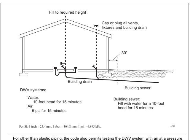
of 5 psi. Pressure air testing of plastic pipe can pose significant safety risks on account of the stored energy of the compressed air.
